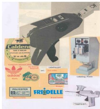
**Fig.3-13: Tagging gun, labelling gun and labelling press**
