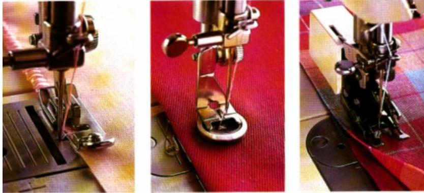
**Fig.4-7: Even feed, button and over edge feet**
